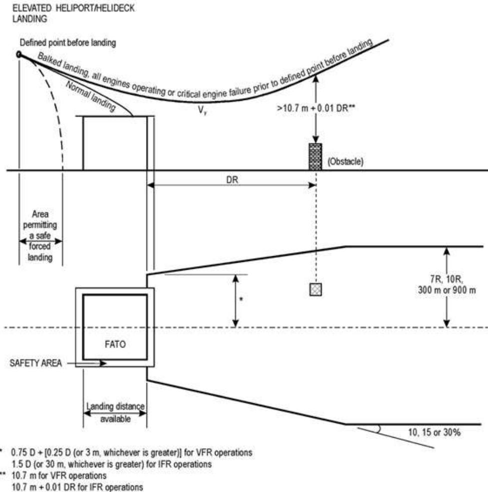
**Figure F-9. Elevated Heliport/Helideck Landing Performance Class 2.**
