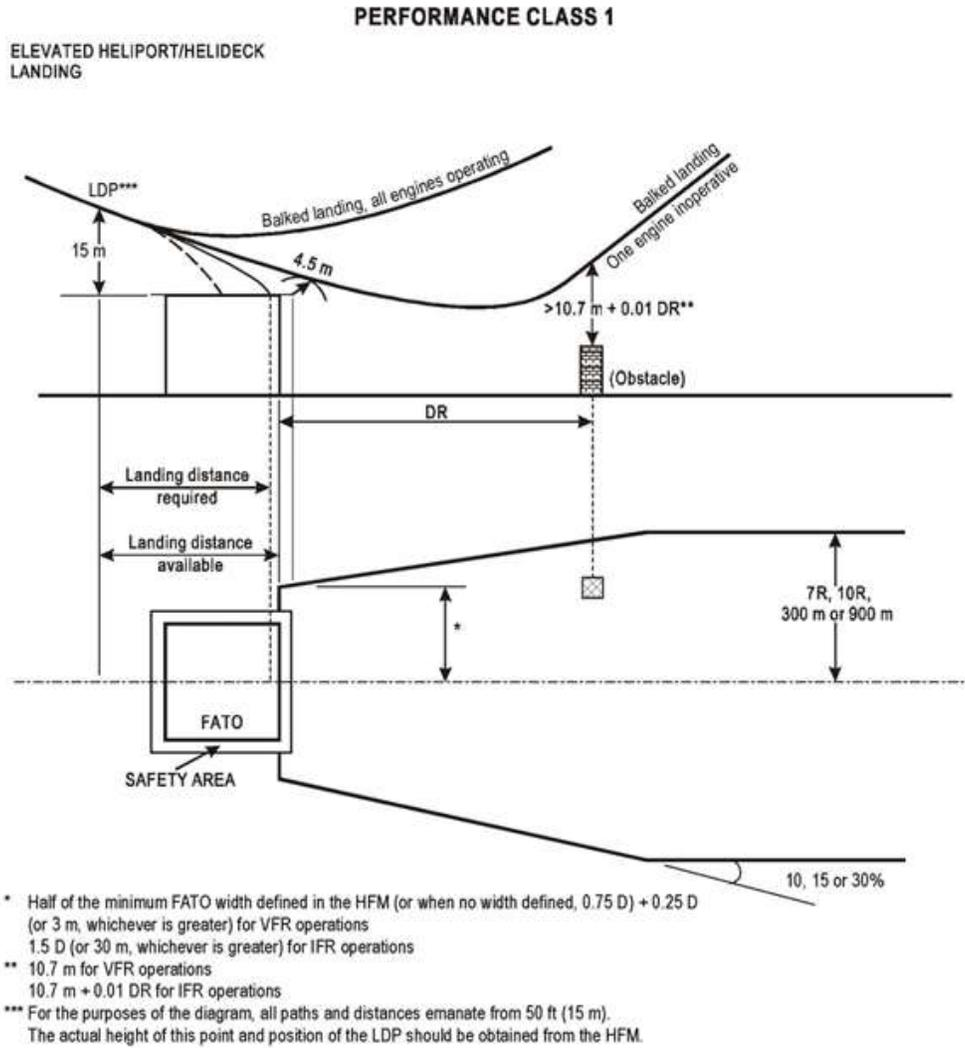
**Figure F–5. Elevated Heliport/Helideck Landing Performance Class 1.**
