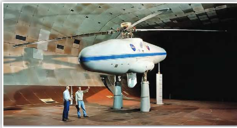
NASA have been recently experimenting in-flight blade control using large scale wind tunnel.
