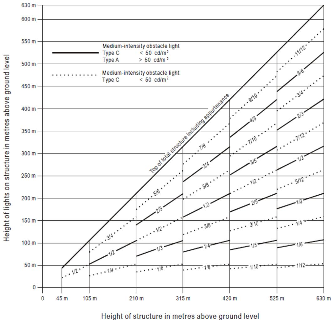
Note. High-intensity obstacle lighting is recommended on structures with a height of more than 150 m above ground level. If medium-intensity lighting is used, marking will also be required.
