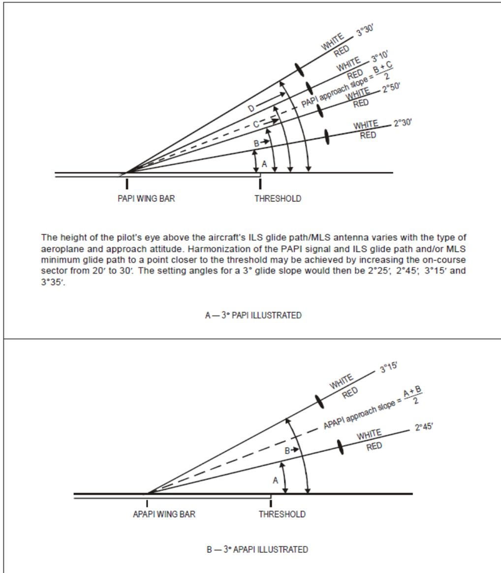
**Figure H-18. Light beams and angle of elevation setting of PAPI and APAPI.**
