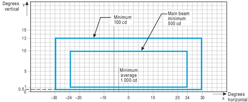
1. Although the lights flash in normal operation, the light intensity is specified as if the lights were fixed for incandescent lamps.
