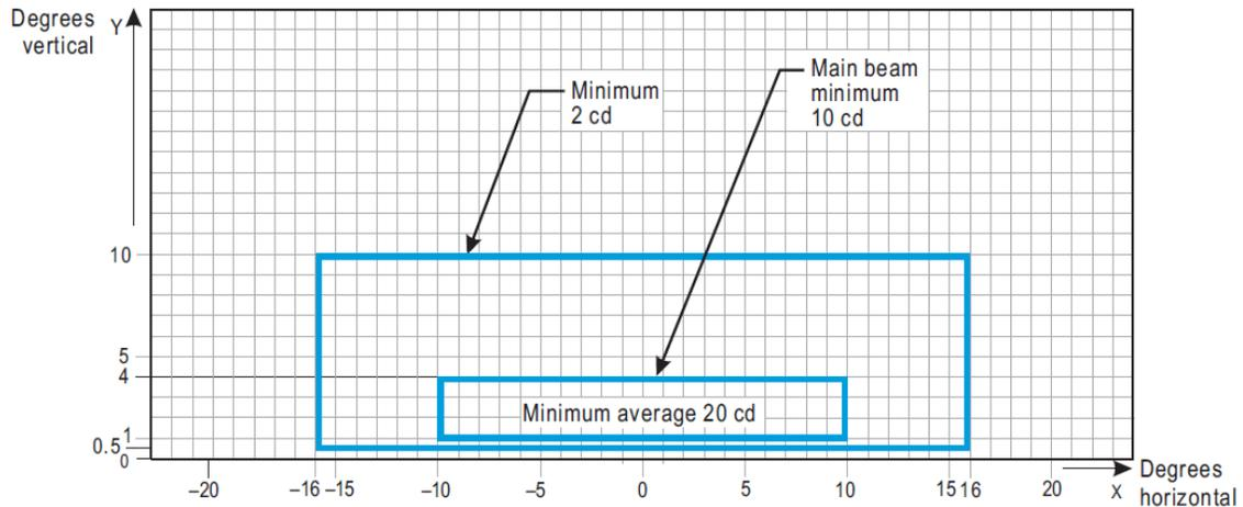
1. At locations where high background luminance is usual and where deterioration of light output resulting from dust, snow and local contamination is a significant factor, the cd-values must be multiplied by 2.5.
