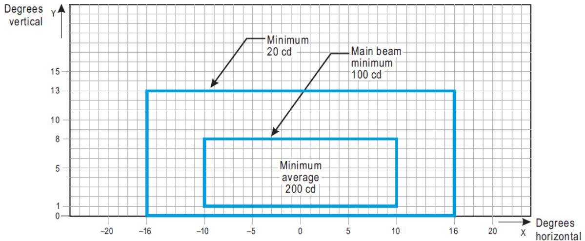
1. These beam coverages allow for displacement of the cockpit from the centre line up to distances of the order of 12 m and are intended for use before and after curves.
