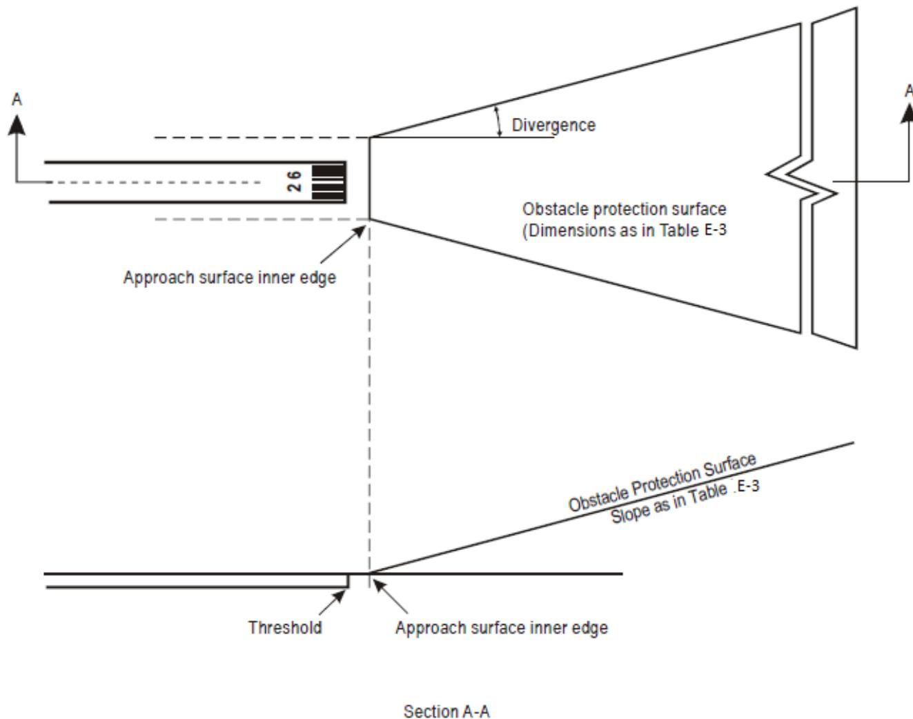
**Figure H-19. Obstacles protection surface for visual approach slop indicator systems**
