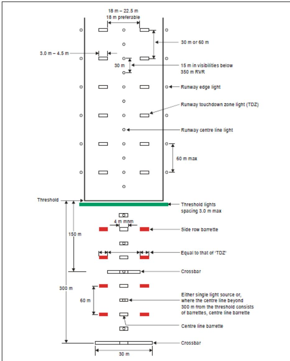
**Figure H-15. Inner 300m approach and runway lighting for a precision approach runway, Categories II and III, where the serviceability levels of the lights specified as maintenance objective in Subpart M can be demonstrated.**
