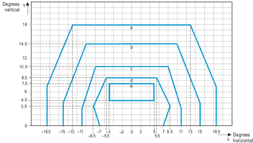
1. Beam coverage is generally satisfactory and caters to a normal displacement of the cockpit corresponding to the outer main gear wheel on the taxiway edge.
