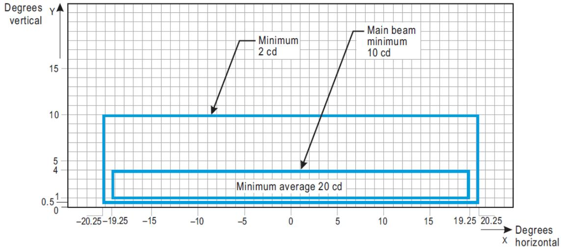
1. Lights on curves to be toed-in 15.75 degrees with respect to the tangent of the curve.
