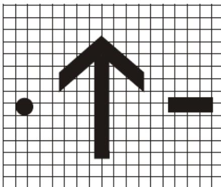
Note 1. The arrow stroke width, diameter of the dot, and both width and length of the dash must be proportioned to the character stroke width.
