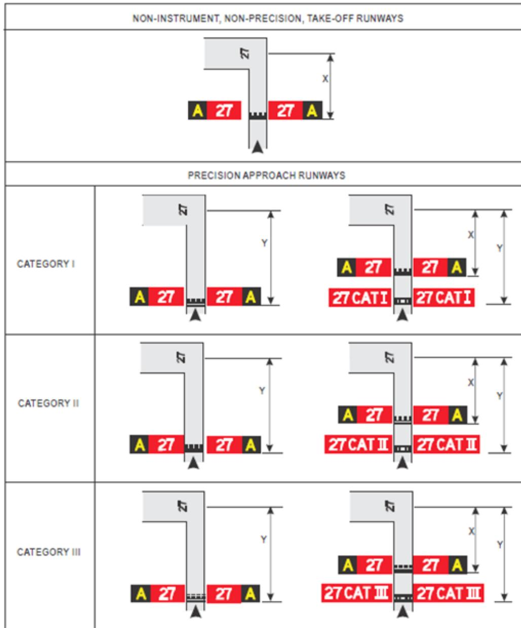
*Note.— Distance X is established in accordance with Table F-2. Distance Y is established at the edge of the ILS/MLS critical/sensitive area.*
