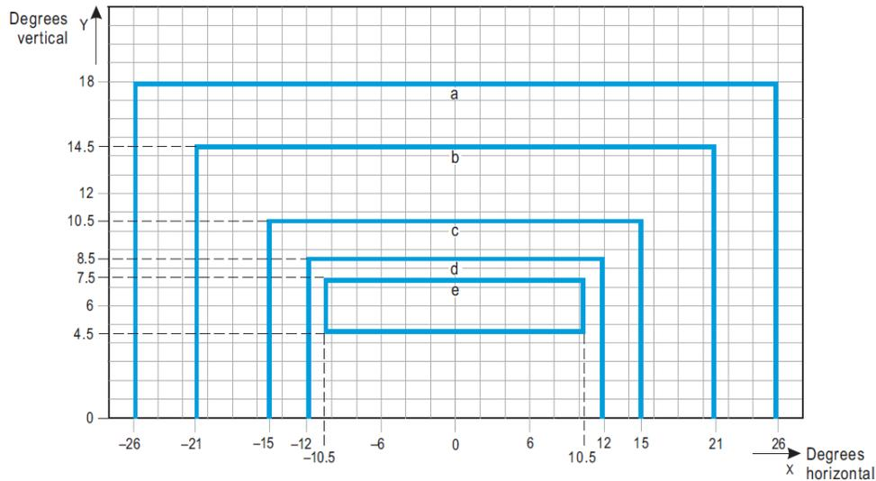
1. Beam coverage allows for displacement of the cockpit from the centre line up of distances in the order of 12 m and is intended for use before and after curves.
