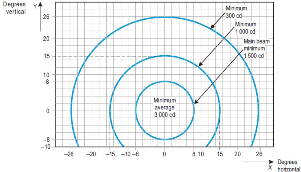
1. Although the lights flash in normal operation, the light intensity is specified as if the lights were fixed for incandescent lamps.
