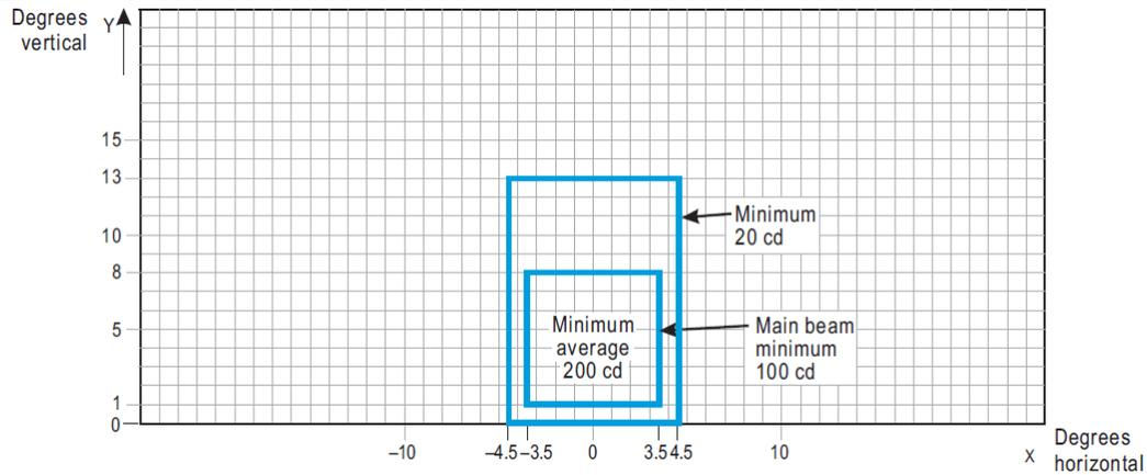
1. These beam coverages are generally satisfactory and cater for a normal displacement of the cockpit from the centre line of approximately 3 m.
