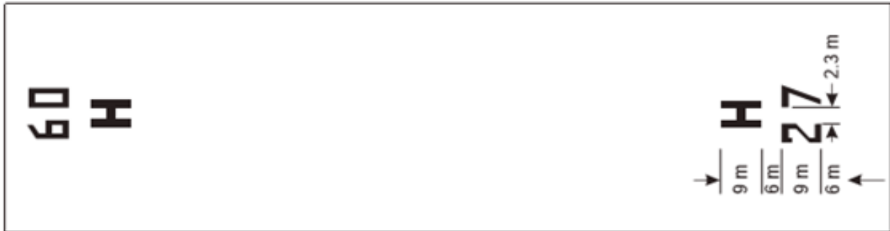
Figure H-2. FATO designation marking and heliport identification marking for a runway-type FATO
